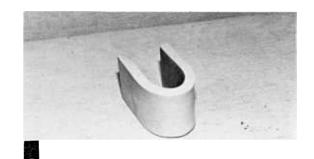
Fig. 57 sawed with the grain, 1/2 inch wide, no welding was done. They were bent double and then pressed flat. Neither of them cracked. That is ductile.
