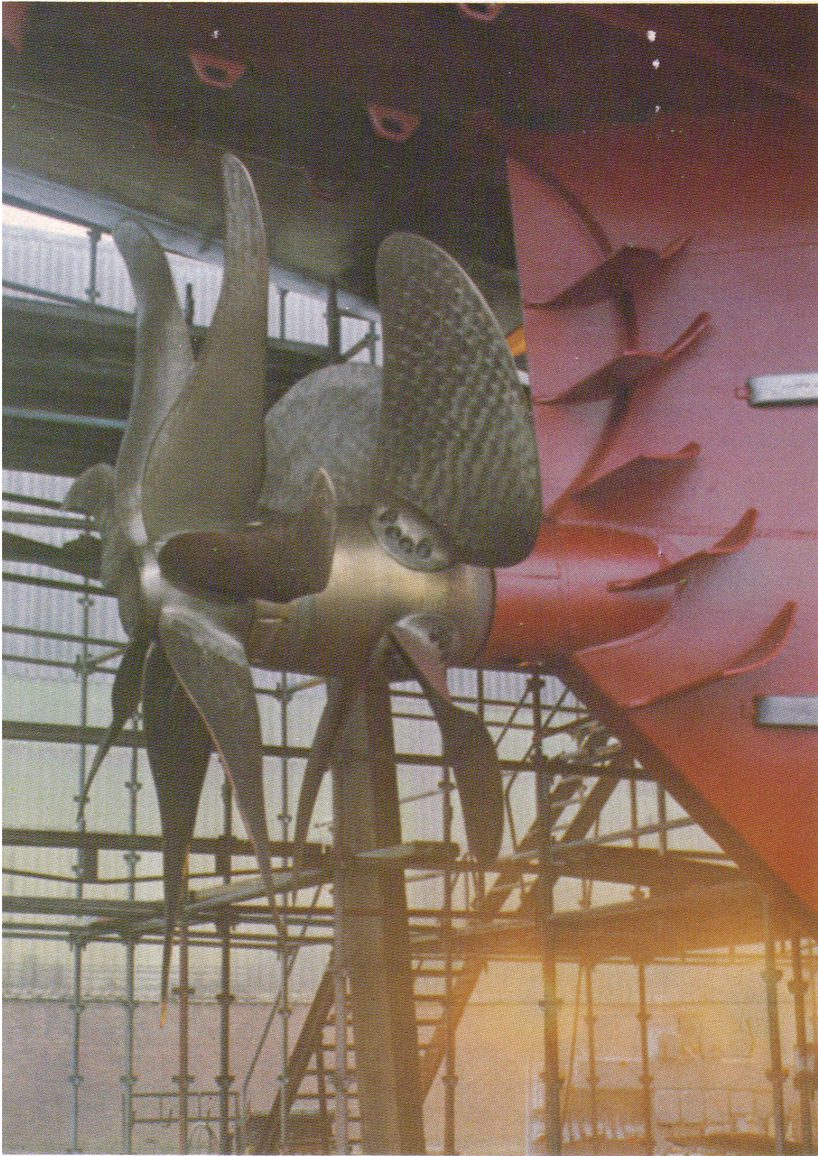
Illustration 20: Grothues spoiler with guide wheel
