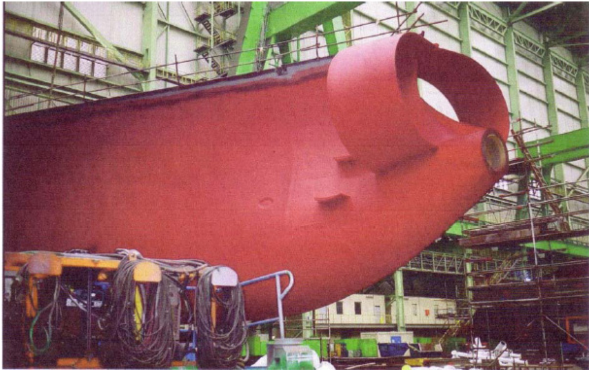
Illustration 17: The Schneekluth WED at the stern
