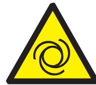
Machinery starts automatically
