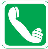
Emergency telephone for first aid or escape
