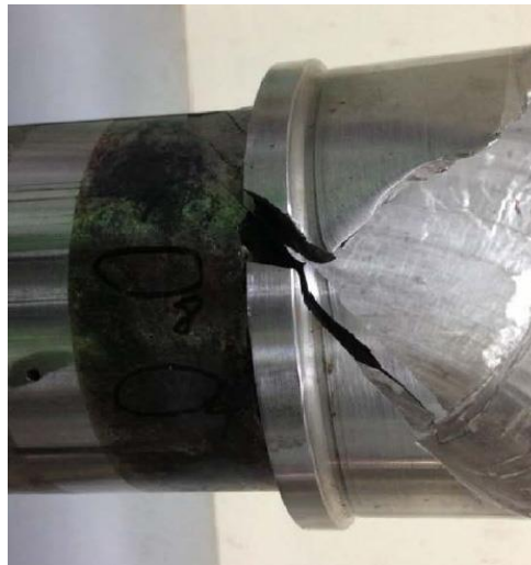
Fig. 2. Shaft crack detail
