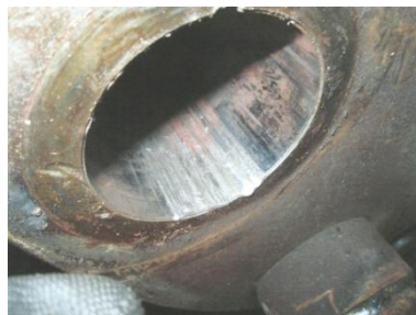
Fig.3 Coupling between intermediate and tail shafts (detail)
