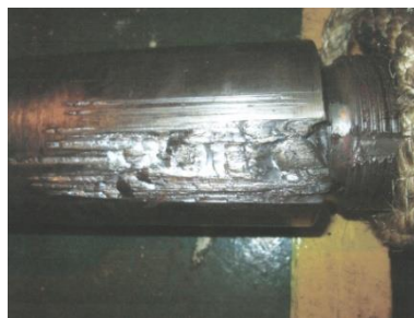
Fig. 2. Coupling between intermediate and tail shafts
